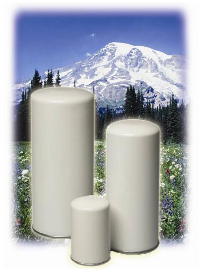
This method of oil separation consists of a deep bed type oil separator element, placed inside of a pressure resistant body, or "can" similar to that of traditional oil filters. Extremely easy to replace in comparison to standard oil-separators which are enclosed in a pressurized tank, this element design is somewhat limited in application due to restrictions of air flow capacity.
