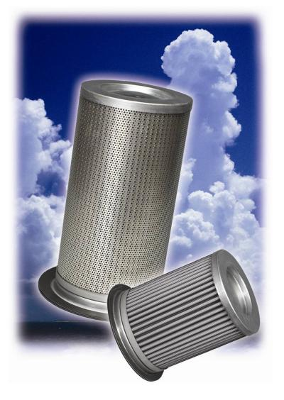
One common method of increasing the capacity of a given sized air-oil separator is through the use of pleated filter media. In this case, the filter media is processed through a machine whereby the normally flat surface is "pleated" or induced into a wave-like appearance. A separator configured in this manner can then be suited for approximately 2x the air flow capacity, as that of a standard air-oil separator, manufactured in the standard, wrapped method.
